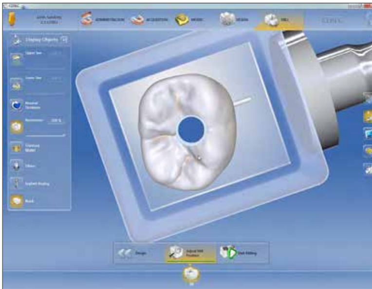
Fig 20: Screw hole location of restoration based on pre-machined hole in e. max block
