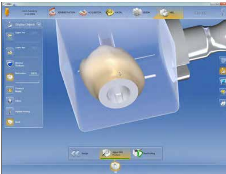
Fig 19: Notch interface relationship to crown (note: e.max block selected is large size to match the AnyRidge large Ti base. The notch and hole are pre-machined into e.max block). For AnyRidge small Ti base/Scan Post, the small e.max block must be selected.
